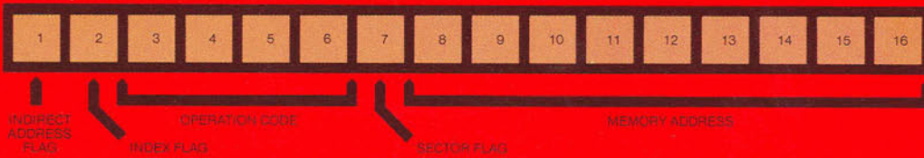
FIGURE 2 INDIRECT ADDRESS FORMAT (STANDARD)
